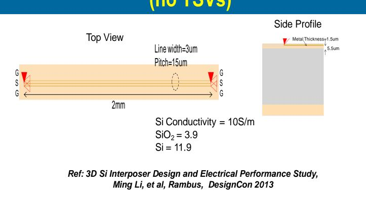
**Analyze: Insertion and Return Losses for GSG structure**
