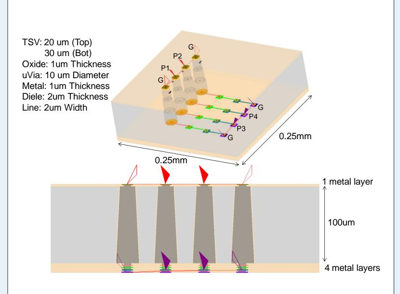
Analyze effect of tapered TSV, RDL, microvias and pads on insertion loss and coupling for a single IC
