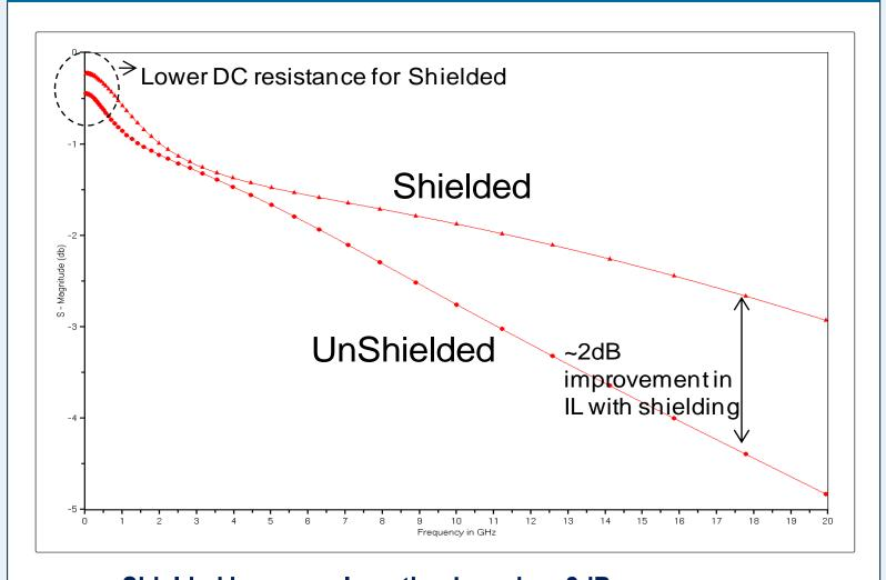
Shielded improves Insertion Loss by ~2dB Lower DC resistance for Shielded
