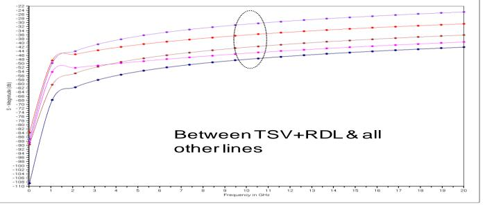
In spite of the ground shield using multiple TSVs, the coupling can still be high. In this example the coupling is between -24 to -48 dB.
