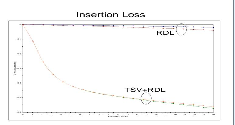
RDL for this structure has minimal IL degradation since they are routed above or below silicon substrate, while TSV/RDL paths have ~14X worse IL
