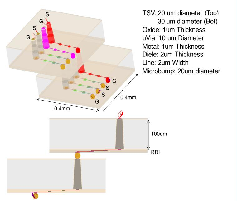
Analyze impact of stacking 2 IC blocks with TSV and solder bumps: Insertion loss and Xtalk
