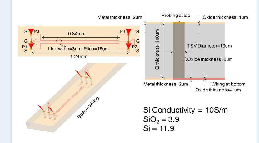
**Analyze: Impact of Si Conductivity on Insertion Loss?**
