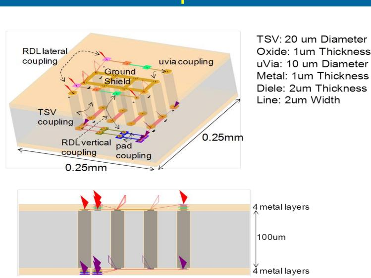
Analyze considerable coupling in spite of ground shield. Ground shield is in the form of grounded TSVs
