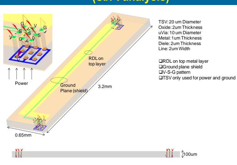
Analyze the coupling between signal and power distribution
